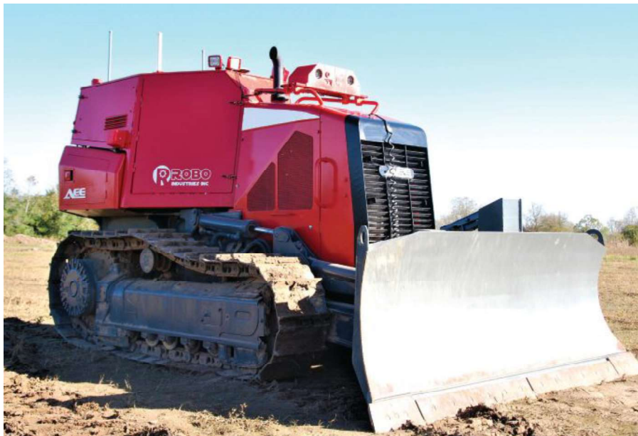
A fully autonomous construction vehicle.
